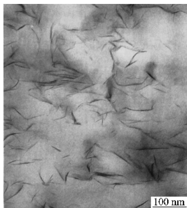
Fig. 3 The typical TEM image of PS/VC_{18} -MMT nanocomposite. The content of MMT is 5\% .
